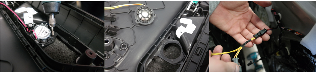
Step 4: Removing the OEM tweeter using a milling cutter (e.g. Dremel)
